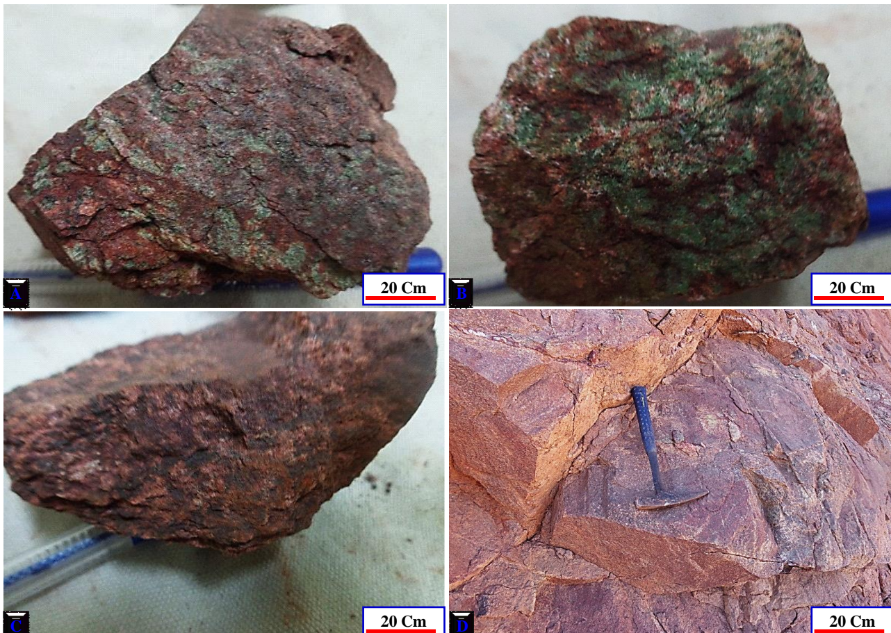
Fig. 7: A, B: Hand samples of the reddish-green slightly weathered crystalline mafic rocks (quartz diorite and gabbro); C: Mottled highly altered rocks of interlocked red-brown and blood red domains; D: Highly altered homogenous rock of massive to argillaceous nature and rich in iron
