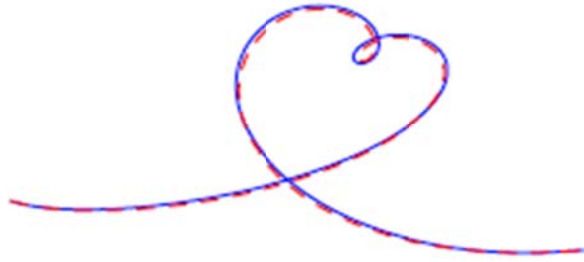
Fig. 3: The corresponding degree reduced Bézier curve using G^2 (Solid-Red)
