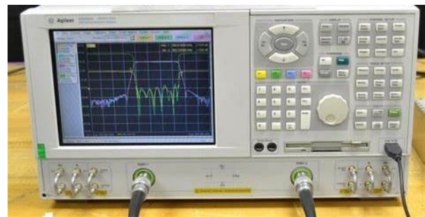
Fig. 2: Experimentation setup of transmission/reflection method
