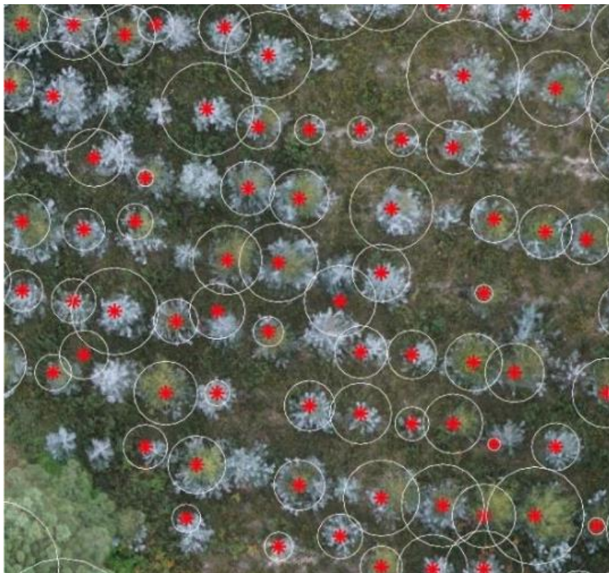
Fig. 3: Trees identified with the estimated crown diameters; trees are represented by red dots
