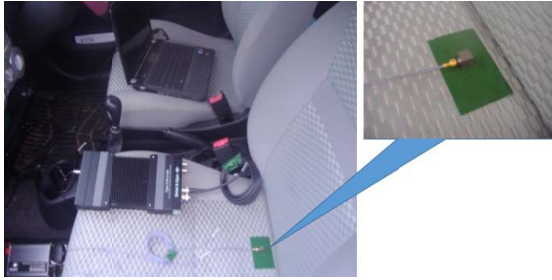
Fig. 5: Accelerometer on the seat
