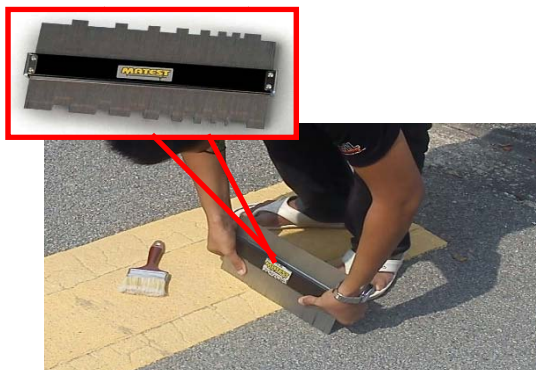
Fig. 6: Barton comb profile meter to measure the TRS thickness
